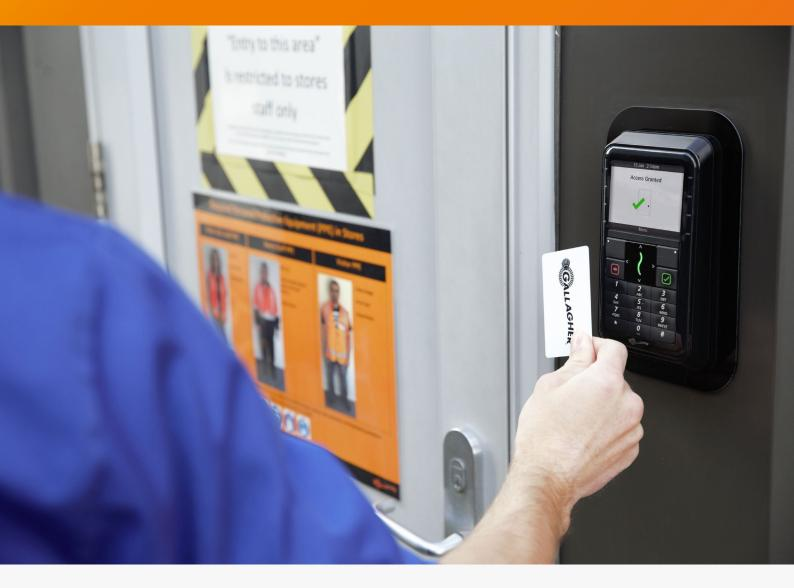
Gallagher's Action on Access solution allows an operator to configure a set of sophisticated access rules. These rules can be used to automate when, where, and why a cardholder can access an area.
